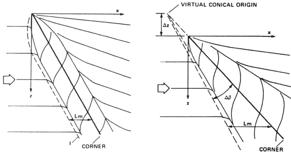
Figure 15. Schematic representations of the surface flow patterns produced by (a) swept compression, and (b) sharp-fin interactions.<sup>21</sup>
