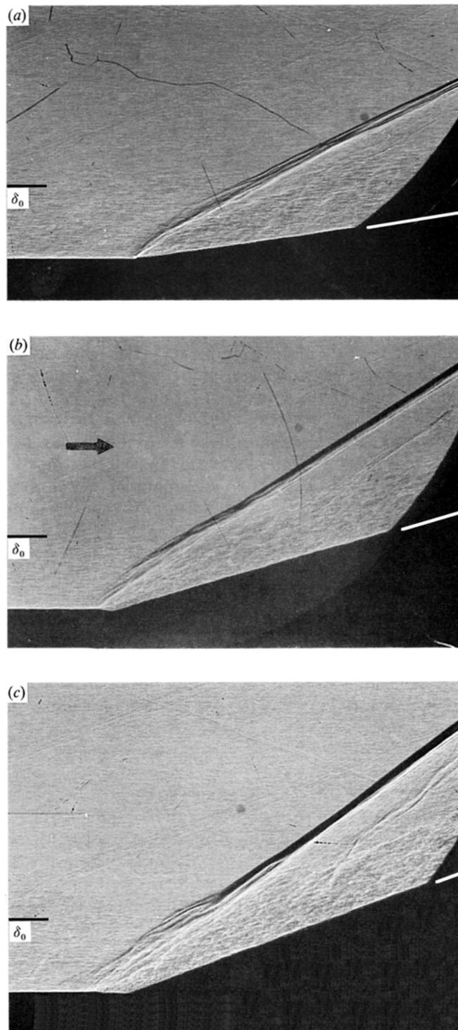
Figure 7. Shadowgraphs of compression corner interactions at a Mach number of 2.9 with turning angles of  $8^\circ$ ,  $16^\circ$ , and  $20^\circ$ . The curved boundaries on the left and right of the pictures are the edges of the circular window, not parts of the model.<sup>48</sup>
