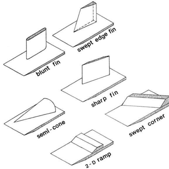
Figure 14. Examples of two- and three-dimensional shock wave-boundary layer interaction geometries studied in the Gasdynamics Laboratory.<sup>27</sup>
