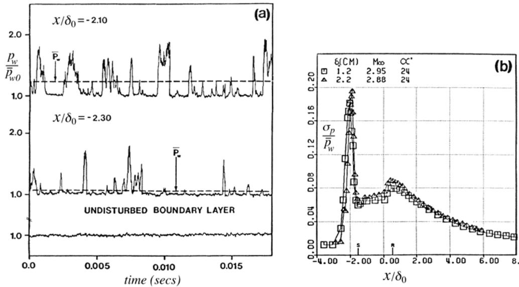
Figure 11. (a) Wall pressure time histories, and (b) *rms* wall pressure levels, in a  $24^\circ$  compression ramp at Mach 3. The lines of mean separation and reattachment are marked by *S* and *R*, respectively. The pressures were non-dimensionalized using the upstream mean wall pressure,  $\bar{p}_{w0}$ ;  $\sigma_p$  is the *rms* wall pressure level.<sup>40</sup>
