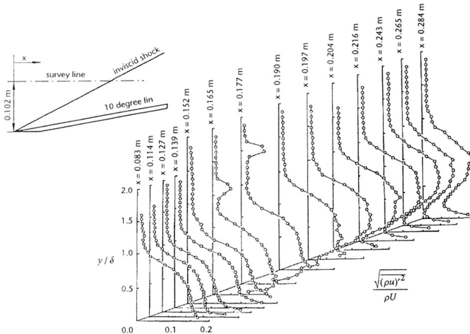
Figure 18. The evolution of the *rms* mass flux intensities for a 10° sharp-fin interaction at Mach 2.9. Data from Tran and Tan (unpublished). (Figure from Konrad.<sup>12</sup>)
