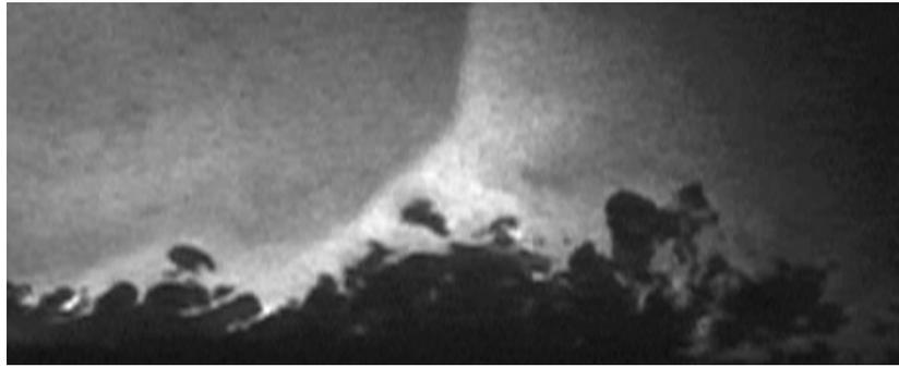
Figure 17. Filtered Rayleigh scattering image of a sharp-fin interaction at Mach 8, with  $Re_\theta = 2400$ . The view is in a plane aligned with the incoming flow direction. Incoming flow is from left to right. Within the interaction, the flow is out of the page at approximately  $16^\circ$ .<sup>2</sup>
