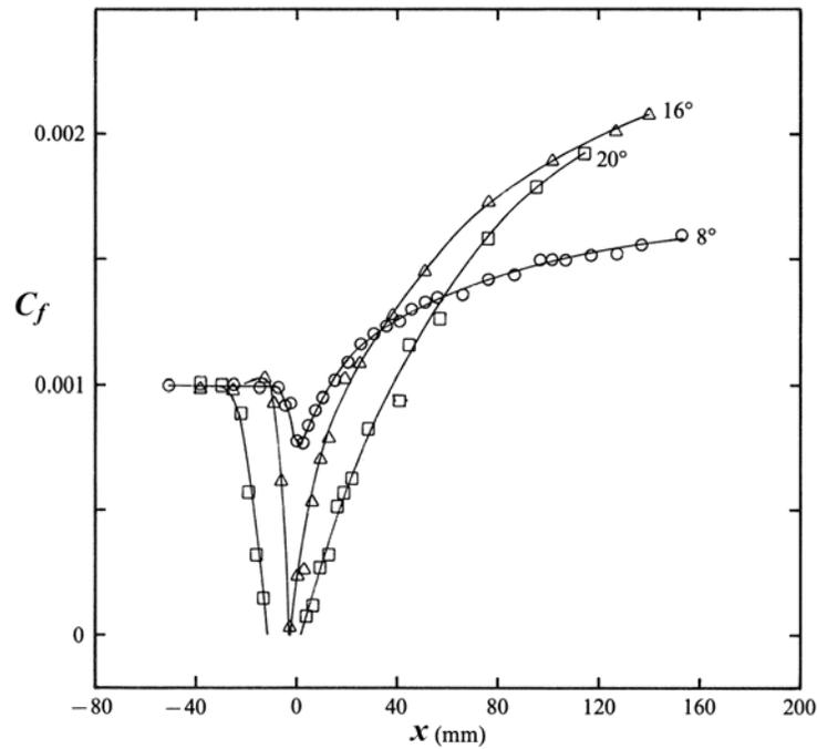
Figure 9. Distributions of  $C_f$  in compression corner interactions at Mach 2.9. The wall stress is non-dimensionalized using “effective” edge conditions based on tunnel stagnation and local static pressures. (Figure adapted from Smits,<sup>24</sup> showing data by Settles.<sup>48</sup>)
