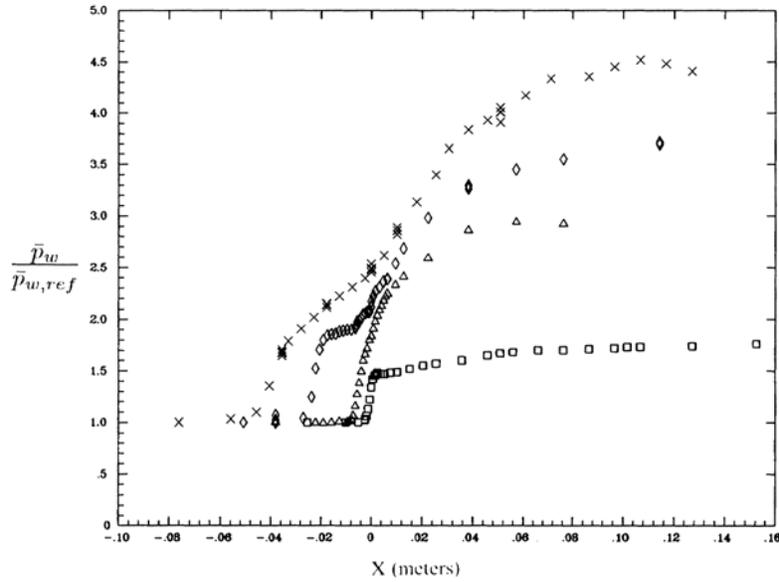
Figure 8. Pressure distributions in compression corner interactions at  $M = 2.9$ :  $\square$ ,  $8^\circ$ ;  $\triangle$ ,  $16^\circ$ ;  $\diamond$ ,  $20^\circ$ ;  $\times$ ,  $24^\circ$ . The pressures are normalized by the value of the wall pressure measured upstream of the interaction, and the distance  $x$  is measured from the start of the compression corner.<sup>48</sup>
