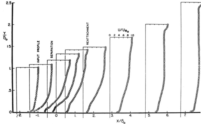
Figure 10. Development of the mean velocity profiles through a  $24^\circ$  compression corner interaction at Mach 2.9, with  $Re_\theta = 72,100$ . Distances and velocities normalized by upstream values. (Figure adapted from Settles.<sup>51</sup>)
