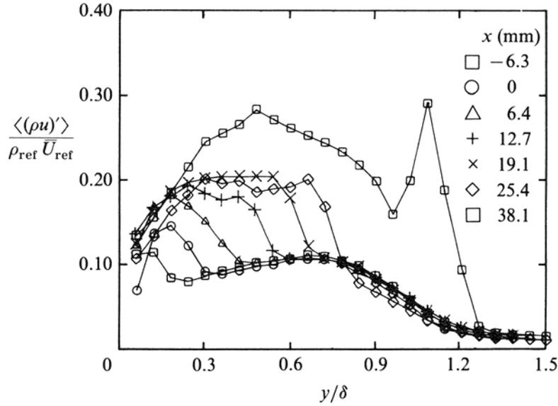
Figure 12. Distributions of  $(\rho u)'$  in  $16^\circ$  compression corner interaction, in the region near the corner.<sup>24</sup>
