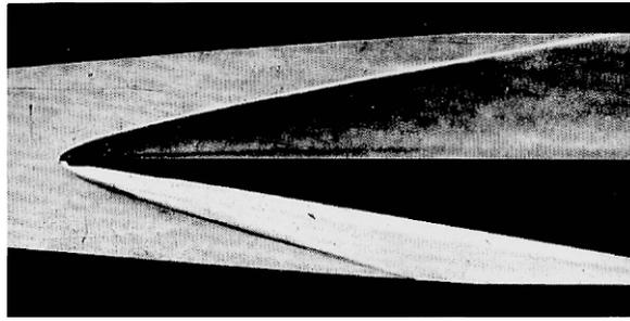
**Figure 6. Schlieren photograph of a blunt flat plate in helium at Mach 11.6. The boundary layer is visible over the top of the plate. The shock shape is close to a power-law shape, with a measured exponent of  $0.66 \pm 0.01$ . This may be compared to the theoretical value by Hayes & Probstein of 0.667. Photo courtesy of the Gas Dynamics Laboratory, Princeton University.**
