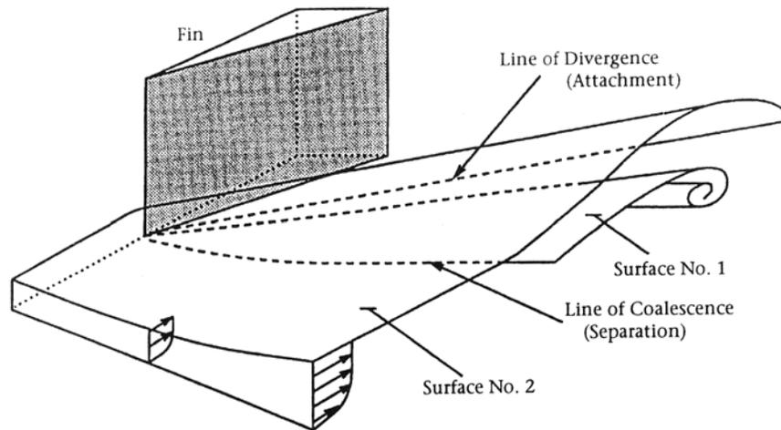
**Figure 16. Structure of three-dimensional shock wave-boundary layer interaction generated by a sharp fin at an angle of attack.<sup>33</sup>**
