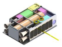
MIT KitCube, 6U CubeSat to demonstrate lasercom, green monopropellant propulsion systems, and 10 arcsec pointing from orbit around the Moon.
